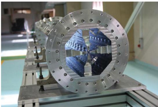
Figure 7: RFQ structure assembly
