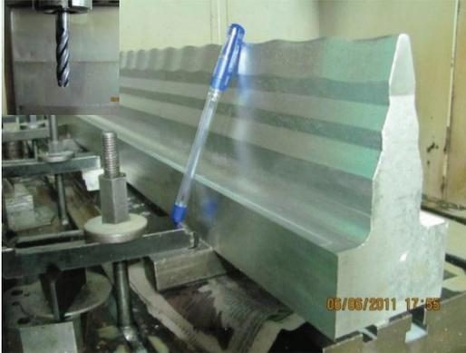
Figure 6: RFQ vane under machining process & cutter used
