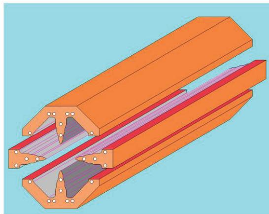
Figure 5: 3D Four joint type fabrication and assembly scheme.
