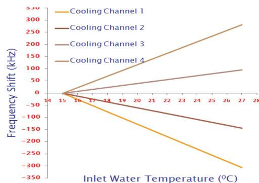
Figure 2: Effect of cooling water temperature on RFQ frequency.
