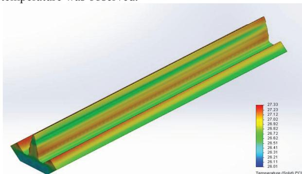
Figure 3: 3D Temperature distribution with counter flow
