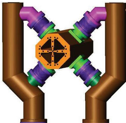
Figure 4: Vacuum envelope for RFQ structure
