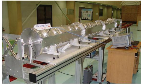
Figure 8: 352.2 MHz prototype RFQ structure assembled on a bead pull test stand
