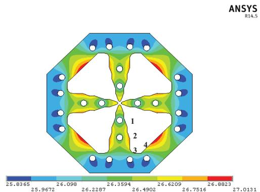
Figure 1: 2D Temperature distribution for RFQ
