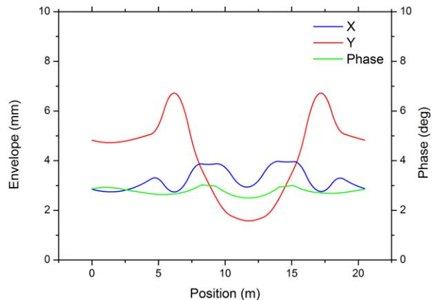
Figure 4: 5\*RMS emittance beam envelopes in a single OSC2 period.
