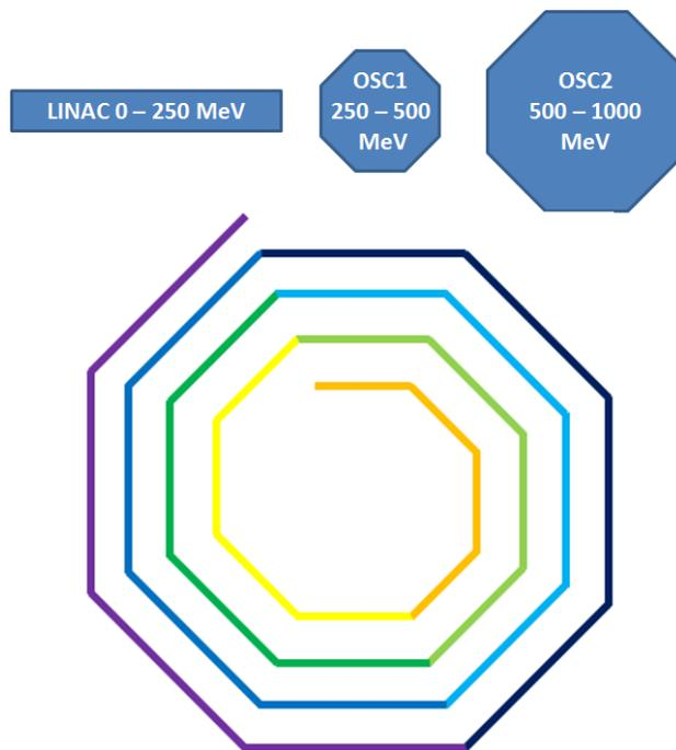
Figure 2: Potential 10 MW accelerator chain (top) and details of the four-turn OSC2 (0.5-1.0 GeV). Colours represent groups of four equal length periods.
