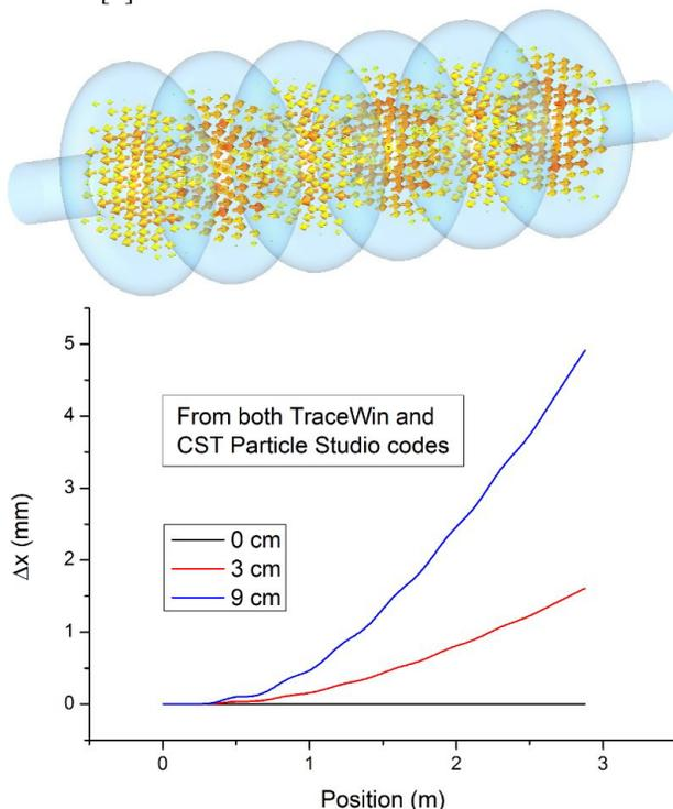
Figure 3: Beam centroid horizontal displacement (bottom) when travelling on and off-axis through a six-cell superconducting RF cavity (top).
