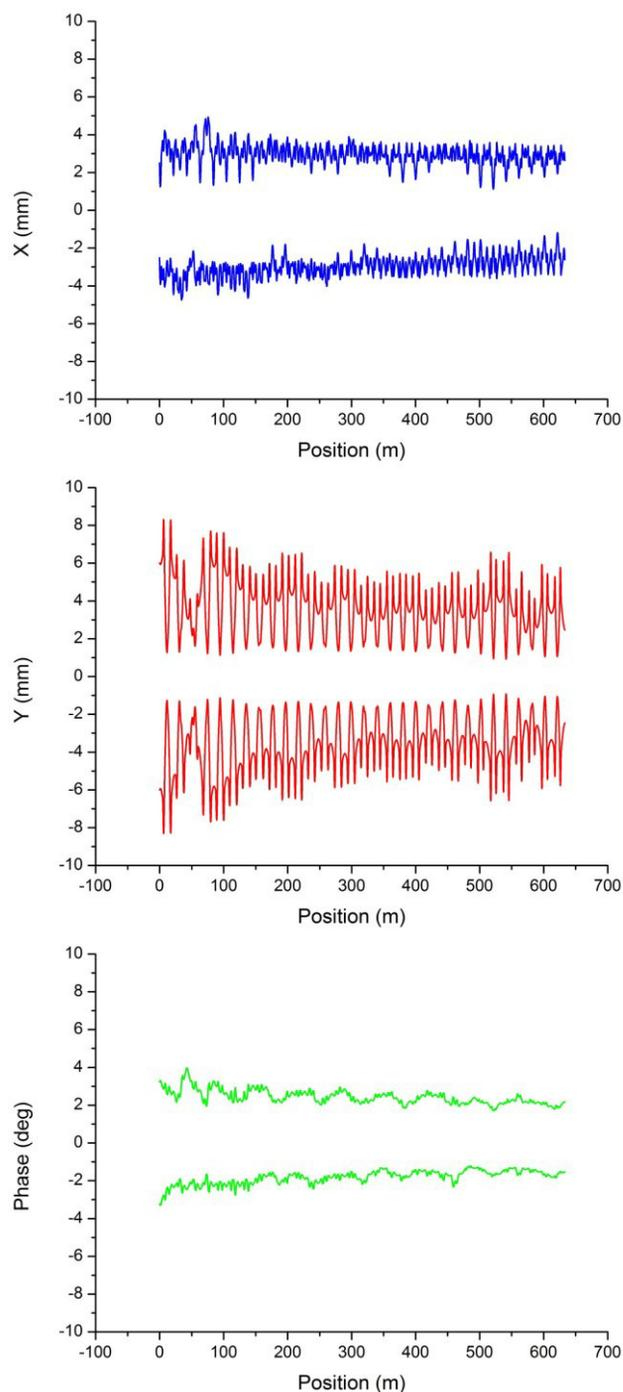
Figure 5: 5\*RMS emittance beam envelopes through OSC2.
