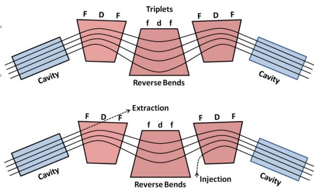
Figure 1: Schematic layout of a typical OSC arc (top), as well as the injection and extraction section (bottom).
