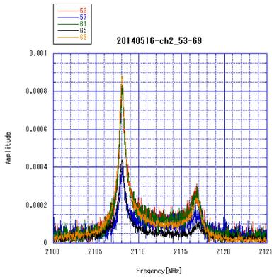
Figure 5-1: Spectrums of Beam Pipe Mode.
