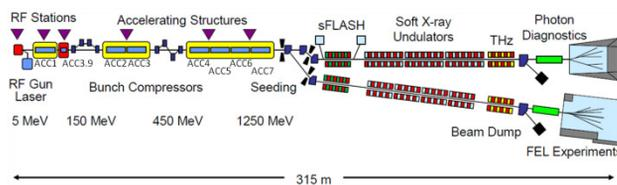
Figure 1: Layout of FLASH accelerator [4].
