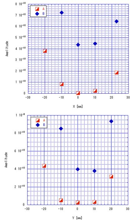
Figure 8: Preliminary result of wire stretched method. The upper plot: wire moved horizontal direction (x). The lower plot: wire moved vertical direction(y).
