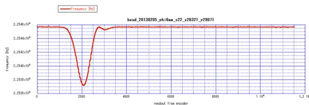
Figure 7: Example of Bead Pull Measurement.
