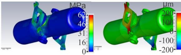
Figure 10: The HWR stress (left) and normal displacement (right) due to 200 μm pretension displacement of both sides of the step motor and piezo and 1.2 bar He pressure.
