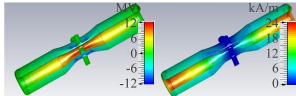
Figure 7: HWR E (left) and H (right) fields.
