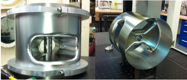
Figure 3: Weld fit-up and completed spoke-outer conductor subassembly
