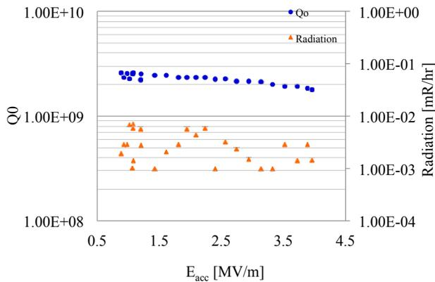
Figure 7: High power test results at 4.3K.
