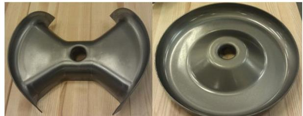
Figure 1: Formed spoke half and end cap.
