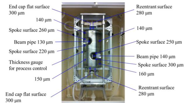
Figure 6: BCP set-up and thickness measurement results.
