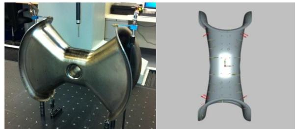
Figure 2: Welded spoke and CMM results showing deviations from the cavity model.
