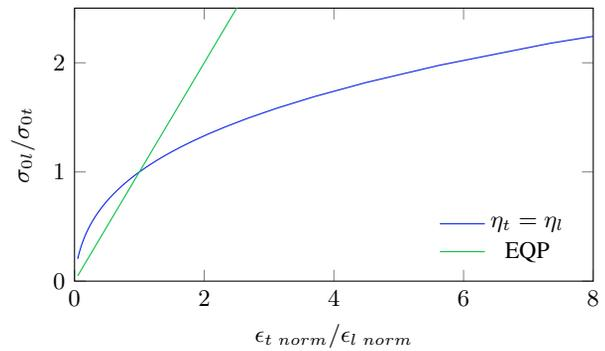
Figure 3: Zero current phase advance ratio as a function of the normalized emittance ratio to satisfy  $\eta_t = \eta_l$ .
