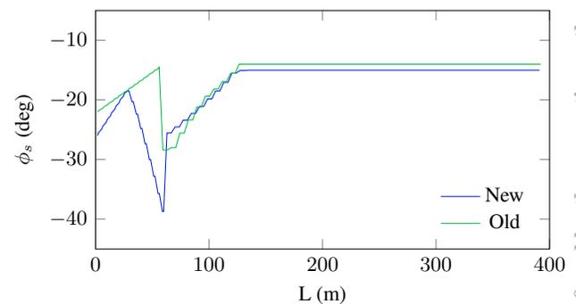
Figure 4: Synchronous phase along the sc linac for the new phase law and the old phase law [24].
