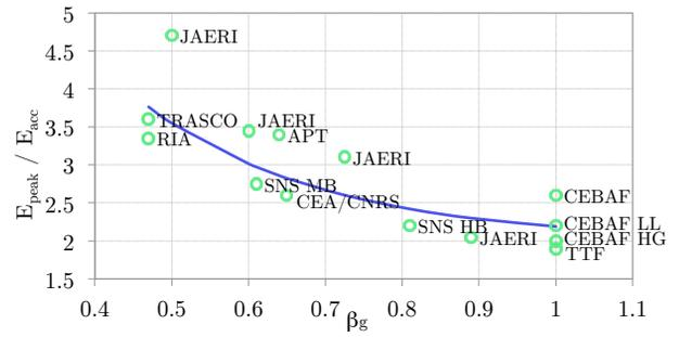
Figure 1:  $E_{peak}/E_{acc}$  as a function of geometric beta [21].
