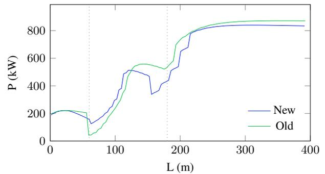
Figure 7: Power delivered to beam per cavity along the sc linac for the new phase law and the old phase law.
