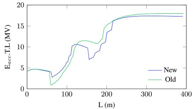
Figure 6: Voltage profile along the sc linac for the new phase law and the old phase law.
