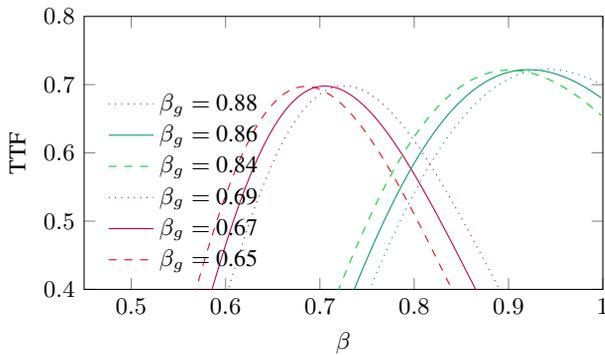
Figure 2: Transit time factor as a function of particle  $\beta$  for different geometric betas. The red series have six cells and the green series are five cell elliptical cavities.
