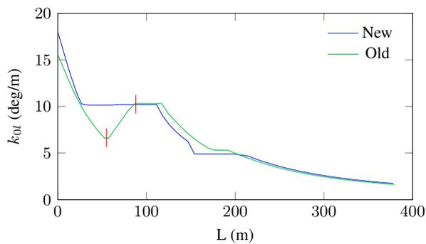
Figure 5: Zero current phase advance along the sc linac for the new phase law and the old phase law.
