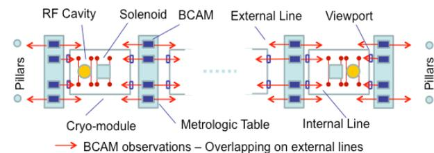
Figure 8: Sketch of the alignment system - Top view.
