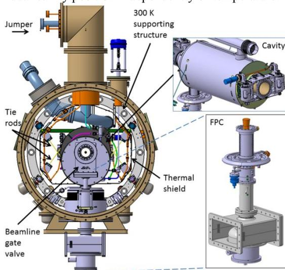
Figure 3: Cross section of a ESS elliptical cryomodules.
