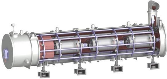
Figure 2: ESS elliptical cavities cryomodules layout.
