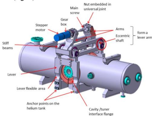
Figure 8: HWR tuner and He jacket layout.
