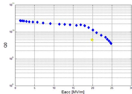
Figure 5: First ESS  $\beta=0.86$  2K VT test result.
