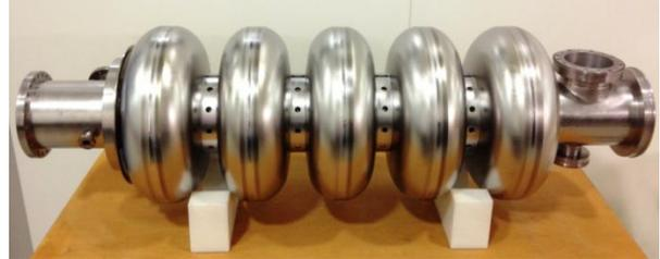
Figure 4: First  $\beta=0.86$  prototype.
