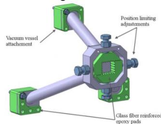
Figure 7: Frame excursion limiting tripod.
