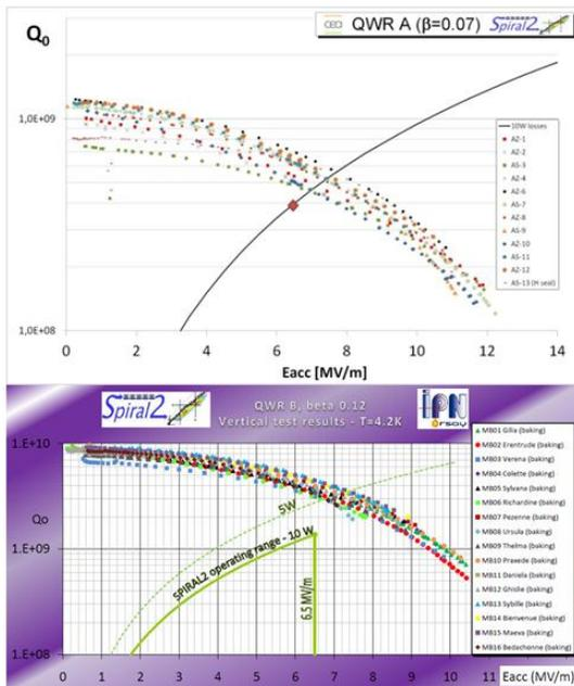
Figure 12 : VT results of QWRs (top : low  $\beta$ , bottom: high  $\beta$ )
