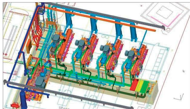
Figure 2: Typical Warm Helium Compressor Layout.
