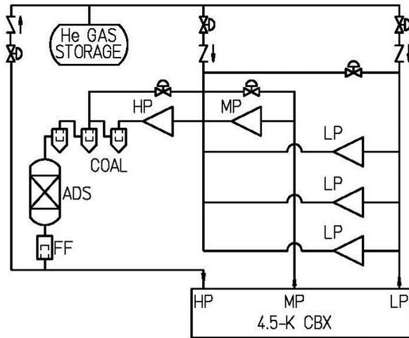
Figure 1: Simplified Warm Helium Compressor System increases at constant pressure ratio. With decreasing load return flow, the charge pressure of the MP and HP stages decreases. Multiple low pressure compressors are provided to process the large cold compressor flow rate during pump down and normal operation of the linac.
