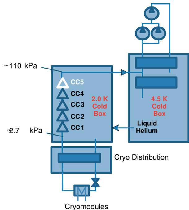
Figure 3: Typical 5 Stage 2K Cold.
