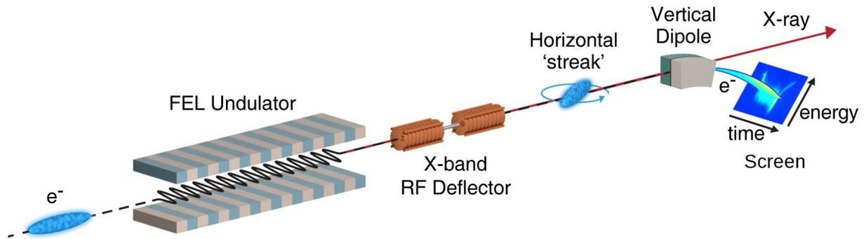
Figure 1: Diagnostic layout of the X-ray temporal measurement. It includes the transverse deflector, the magnetic spectrometer and the Ce:YAG screen located downstream of the FEL undulator. Two 1-m long X-band rf deflecting structures provide horizontal streaking followed by a vertical-bend dipole magnet for measuring the energy spectrum. A camera captures the transverse images of the electron beam density distribution on the diagnostic screen. The plot is from [7].
