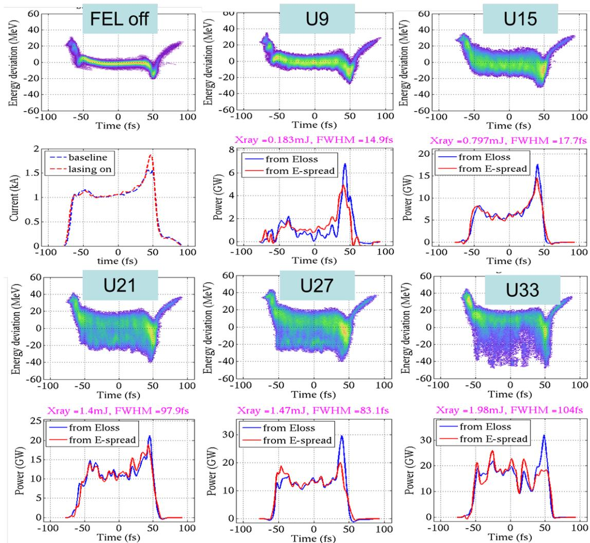
Figure 3: Temporal profile reconstruction. The electron bunch charge is 150 pC with an energy of 4.7 GeV to produce photons at 1.0 keV. The measured single-shot longitudinal phase space images are shown in (a): “lasing off” and (b): “lasing on”. The reconstructed X-ray power profiles are shown in (c) from the time-dependent energy loss (blue curve) and energy spread growth (red curve). The bunch head is to the left in these plots and throughout.
