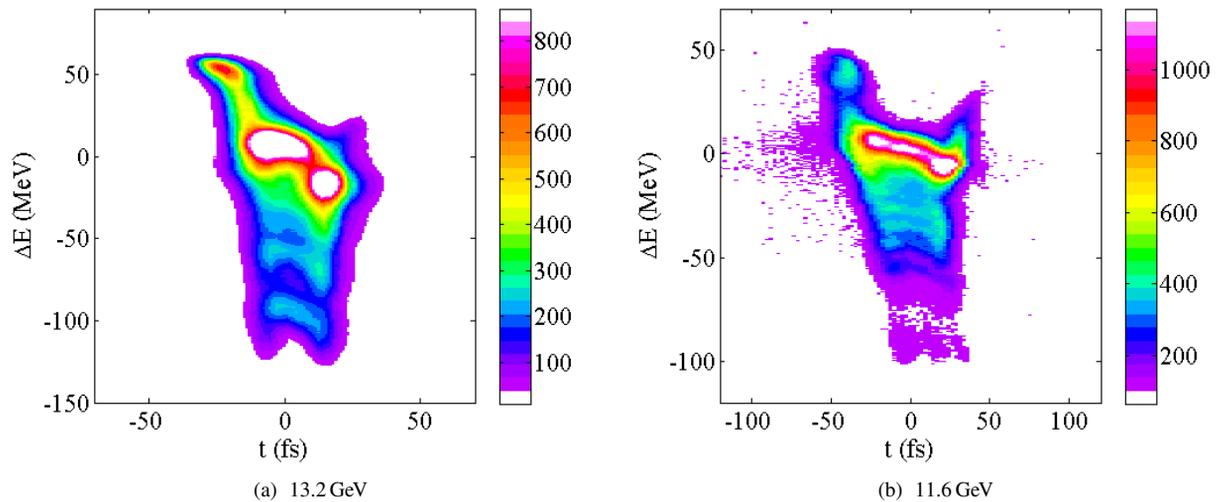
Figure 4: Particle trapping. Measured electron beam longitudinal phase space images at electron energy 13.2 GeV and 11.6 GeV, at the end of the undulator. The isolated energy stripes from the trapping feature are clear at the low energy side of the phase space. We used a special color map from F. - J. Decker to enhance the visibility of the trapping [20].
