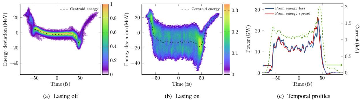
Figure 2: Temporal profile reconstruction. The electron bunch charge is 150 pC with an energy of 4.7 GeV to produce photons at 1.0 keV. The measured single-shot longitudinal phase space images are shown in (a): “lasing off” and (b): “lasing on”. The reconstructed X-ray power profiles are shown in (c) from the time-dependent energy loss (blue curve) and energy spread growth (red curve). The bunch head is to the left in these plots and throughout. The plots are from [7].
