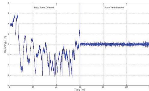
Figure 7: PZT off vs. on.
