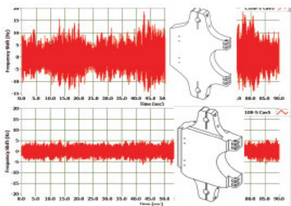
Figure 6: Time domain microphonics data before and after tuner modification.
