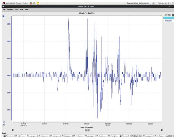
Figure 8: Showing He liquid level in a cryomodule when the resistive heaters are turned on.
