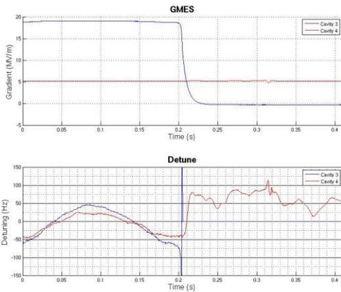
Figure 5: Graph of gradient and detuning (Hz) as a cavity is faulting (blue).
