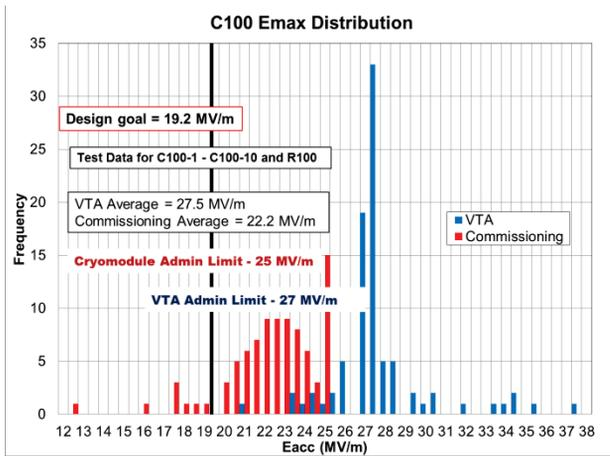
Figure 1: Emax distribution between the installed cavities and data taken during cavity vertical test.
