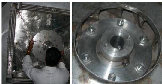
Figure 4: Heat exchanger assembly and blower inside accelerator tank
