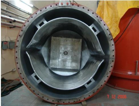
Figure 5: Rectangular Radiator type Heat Exchanger with Blower assembled inside the Accelerator Tank
