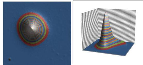
Figure 5: Beam footprint with octupoles off/on (left/right). Transverse coupling is visible in the footprint with couple off (left)
