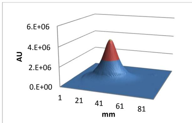
Figure 4: Beam footprint at the BLIP target for 130- $\mu$ A-beam current.
