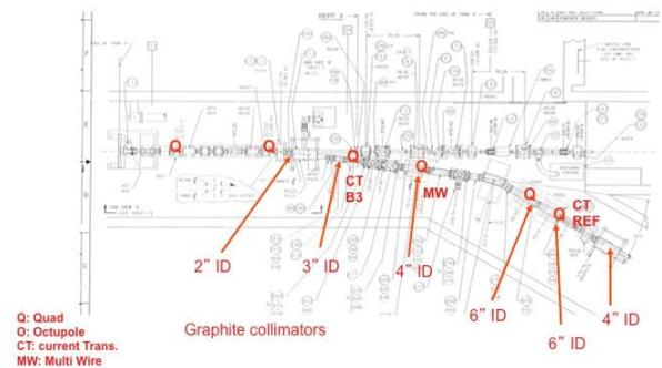
Figure 1: Layout-1 of the BLIP line showing quadrupoles (Q), octupoles (O), dipole magnet (D) and profile monitors.
