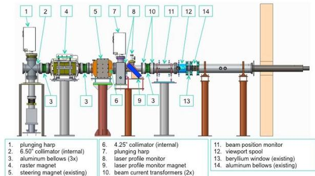
Figure 9: Proposed lay out of the last leg of the BLIP beam line.
