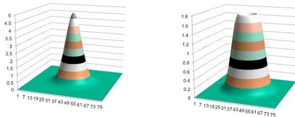
Figure 8: (left) Gaussian beam with FWHM of 18 mm, (right) raster beam as describe in Figure 6. Ordinate is in same arbitrary unit.
