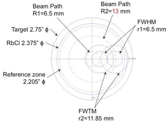
Figure 7: Raster scheme for BLIP. A 6.5 mm (FWHM) beam paint in circular fashion at radius of 13 mm for 4 pulses and 5<sup>th</sup> pulse at radius of 6.5 mm.
