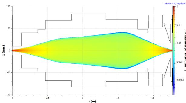
Figure 2: Results of a beam transport simulation: beam density along the LEBT.
