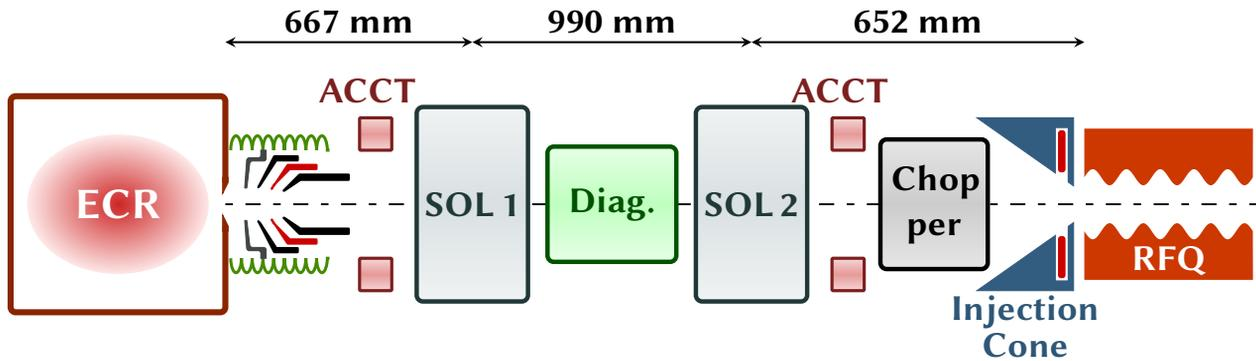
Figure 1: Schematic layout of the FAIR proton linac ion source and LEBT.
