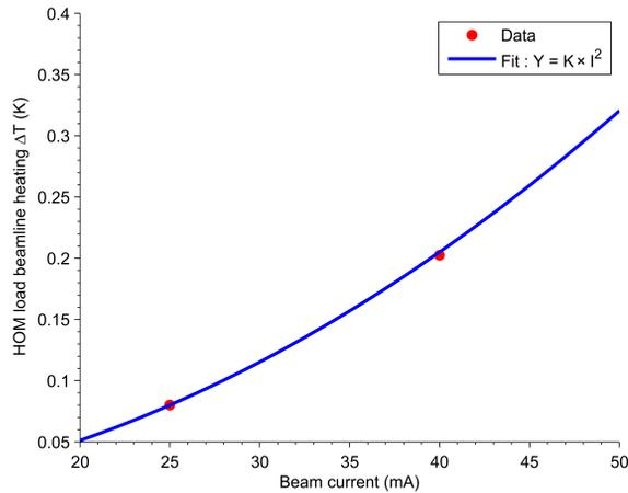
Figure 3: Data taken measuring the rise in temperature of the stainless steel beampipes of the HOM load whose beampipes had not been coated with copper, at 2 different values of beam current and scaled to a bunch length of 2 ps. At 100 mA in an ERL configuration,  $\Delta T = 3$  K.
