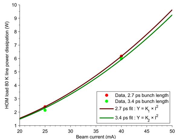
Figure 2: Data taken measuring the power dissipated in the HOM loads at 2 different values of beam current and bunch length. The scaling relation in Equation 1 has been fitted to both sets of data. At 100 mA beam current in an ERL configuration with a 2 ps long bunch,  $P_{load}^{(ERL)} = 90$  W.
