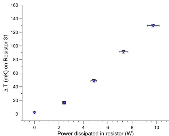
Figure 5: A plot of the temperature difference between the bath and the resistor located above the heater on the steel plate, ΔT, as a function of the power dissipated in the heater. As expected, the dependence between power dissipated and ΔT is linear.
