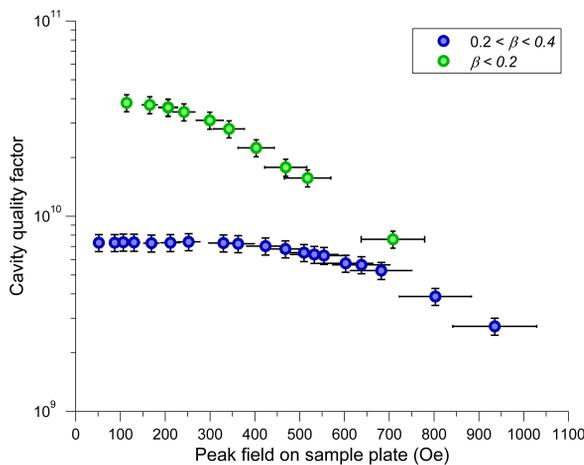
Figure 3: A plot of the quality factor of the cavity against the peak field on the surface of the sample plate, for two different ranges of the coupling β. The lower quality factor observed at higher coupling is due to losses in the coupler.
