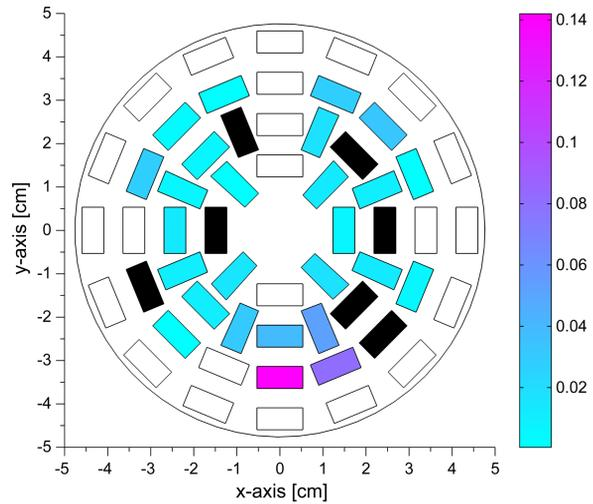
Figure 4: A temperature map of the steel plate equipped with heating resistors. Each box represent a resistor's location on the plate; white boxes indicate a resistor that is either missing (the entire outer ring) or currently unmapped. Resistors in black have failed to calibrate correctly during cooldown to 1.8 K. With a power of 10 W being dissipated in the resistor, the hotspot is clearly visible in the lower section of the temperature map.
