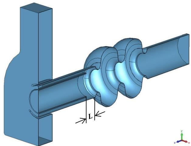
Figure 1: 2-cell cavity with the symmetric coupler.
