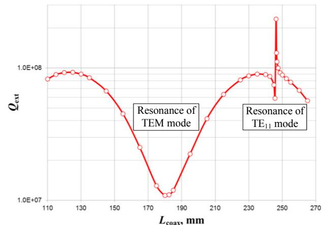
Figure 7: Coupling as a function of the length of the coaxial line for a fixed distance to the cavity.
