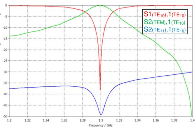
Figure 10: Calculated S-parameters of the improved coupler waveguide-to-coax field transformer (in dB).
