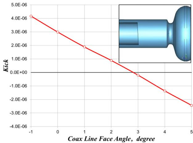
Figure 9: Dependence of transverse kick on cut angle of the coaxial tube.
