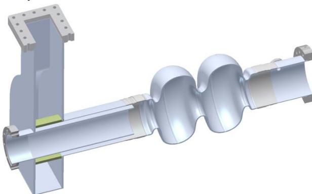
Figure 5: ERL injector cavity with symmetric coupler.
