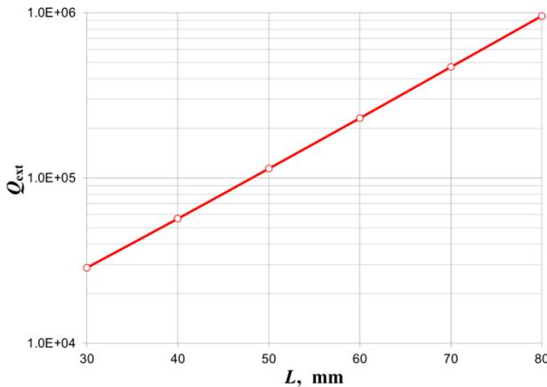
Figure 3: Dependence of coupling on the distance from the cavity to the coaxial line.
