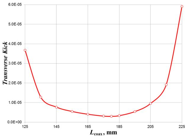
Figure 8: Dependence of kick on the length of coaxial line for a constant  $Q_{\text{ext}}$ .
