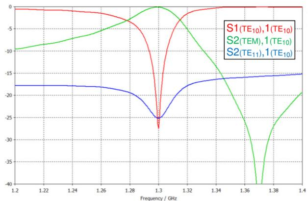
Figure 2: Calculated S-parameters of the coupler waveguide-to-coax field transformer (in dB).
