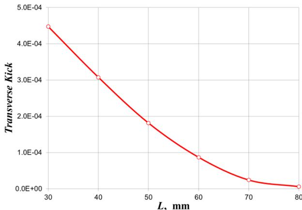
Figure 4: Transverse kick as a function of distance to the cavity.
