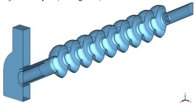
Figure 6: Model of ILC cavity with symmetric coupler.
