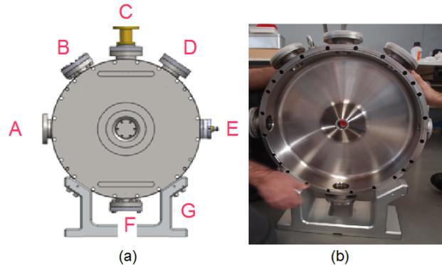
Figure 1: (a) Designed and (b) manufactured cavity.
