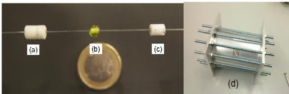
Figure 3: (a) macor ( $\epsilon_r=6$ ), (b) glass ( $\epsilon_r=4.5$ ) and (c) teflon ( $\epsilon_r=2.1$ ) dielectric beads and (d) manufactured pillbox cavity in aluminium (radius = 65 mm, length = 200 mm).
