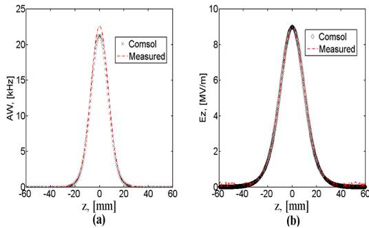
Figure 4: Comparison of the measured and simulated (a) frequency shift  $\Delta\omega$  and (b) the absolute electric field  $E_0$ , as a function of the axial position  $z$  for the teflon bead.
