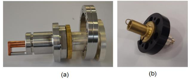
Figure 5: (a) RF coupler for the buncher cavity designed at ESS-Bilbao; (b) LEP pick-up designed by CERN.
