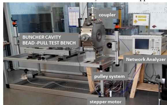
Figure 2: ESS-Bilbao bead-pull test bench design.
