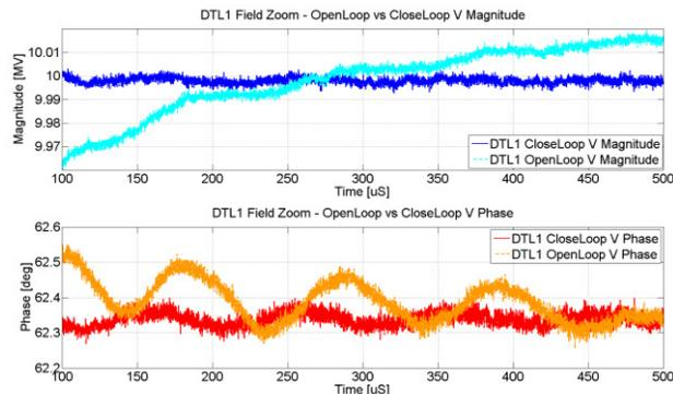
Figure 4: Top: stability of the field magnitude. Bottom: field phase. With regulation (Closed Loop) and without (Open Loop). No beam.
