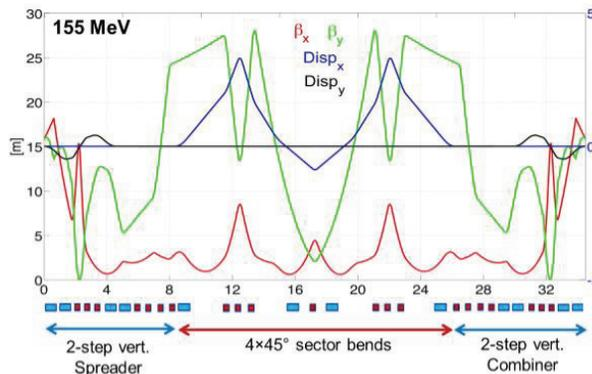
Figure 5: Optics based on an FMC cell of the lowest energy return arc at 155 MeV. Horizontal (red) and vertical (green)  $\beta$ -functions are shown. Blue and black curves show horizontal and vertical dispersion, respectively.
