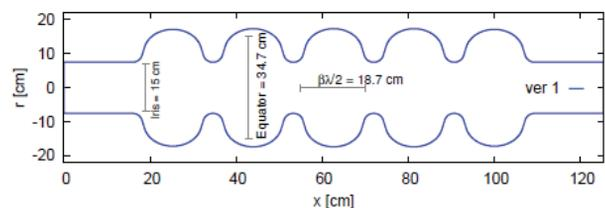
Figure 2: 5-cell cavity envelope for 802 MHz, version 1 with 150 mm aperture.
