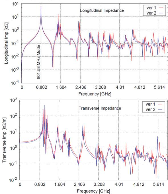
Figure 3: Longitudinal (top) and transverse impedance spectrum of initial 5-cell, 802 MHz cavities. ver 1: 150 mm aperture, ver 2: 160 mm iris aperture.
