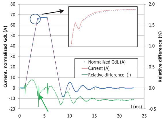
Figure 2: Current and normalized field integral profiles showing the exponential transient due to eddy currents. (highlighted by the green arrow). The insert shows the current overshoot at the end of the ramp-up.
