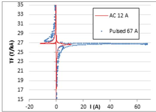
Figure 4: Dynamic integrated gradient transfer function in pulsed and AC excitation modes.
