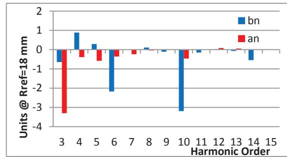
Figure 6: Field harmonics of EMQ 018 at 67.4 A in units of  $10^{-4}$  w.r.t. the main component.
