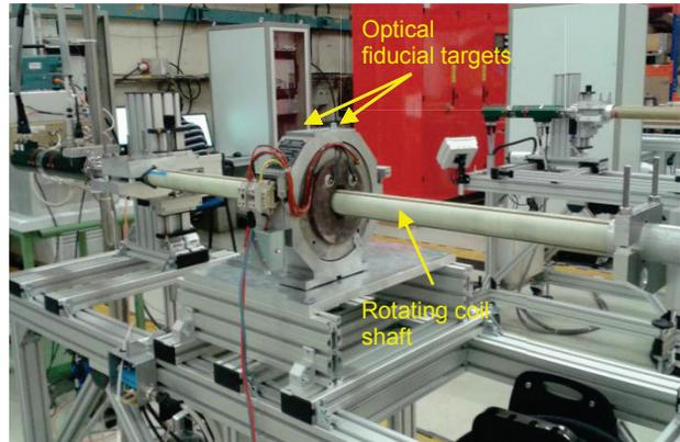
Figure 1: An EMQ on the rotating coil bench.
