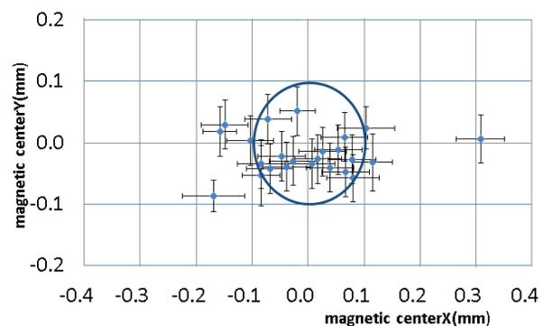
Figure 3: Summary of magnetic axis offset w.r.t. the nominal mechanical axis.
