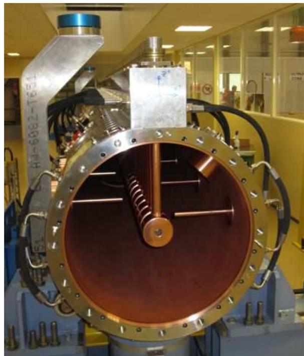
Figure 1: DTL Tank1 assembled.
