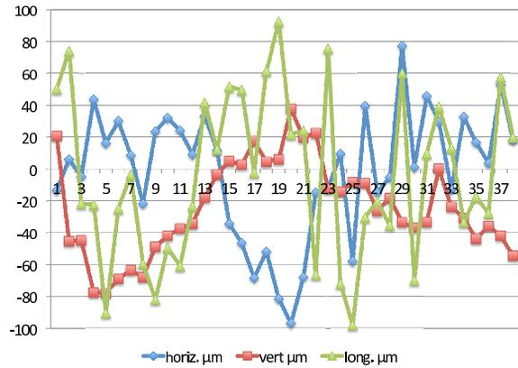
Figure 3: Alignment errors of drift tubes over the whole tank. The interface between the two segments is between drift tube 22 and 23.
