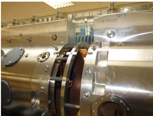
Figure 2: Interface between segments T3S1 and T3S2 before closure with inter-segment ring and key.
