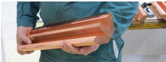
Figure 5: A major vane after rough machining.
