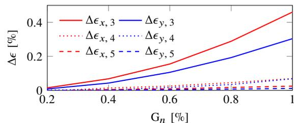
Figure 1: Additional emittance growth due to the multipoles.
