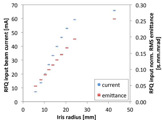
Figure 3: RFQ input beam current and RMS emittance.
