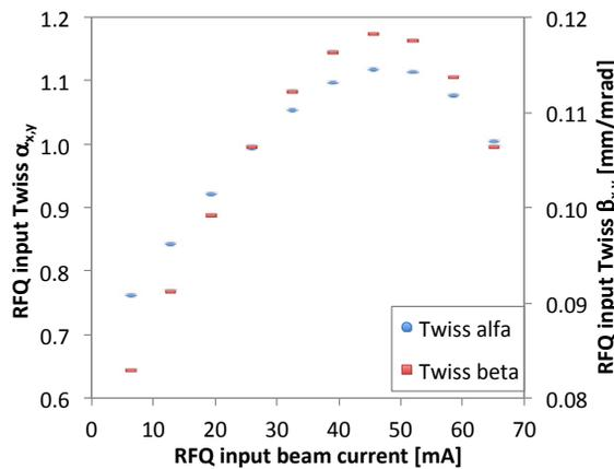
Figure 5: Matched RFQ input beam Twiss parameters.
