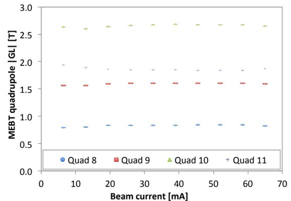
Figure 7: Integrated gradient of the last four MEBT quadrupoles.
