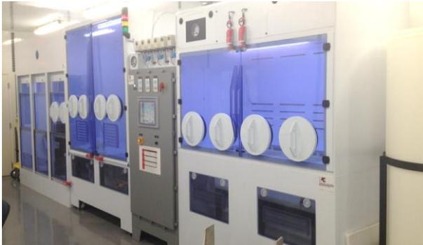
Figure 3: Automated chemical etch tools.
