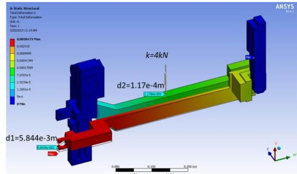
Advantage  $d1/d2 \sim 50$ . Tuner Efficiency = 94%
