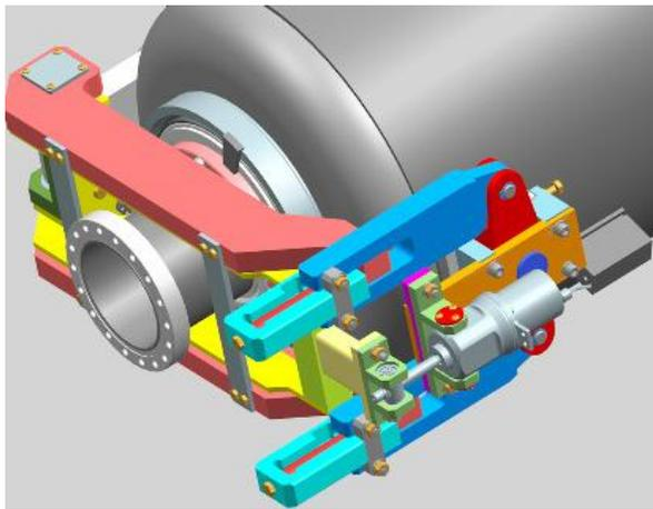
Figure 2: 3-D picture of the tuner. The electromechanical actuator is removable through a special port. The fine/fast tuner consists of two capsules with piezo-actuators installed inside special cartridges. Each of the encapsulated piezoactuators can be replaced through a special port.
