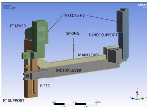
Figure 3: ANSYS model of tuner system.
