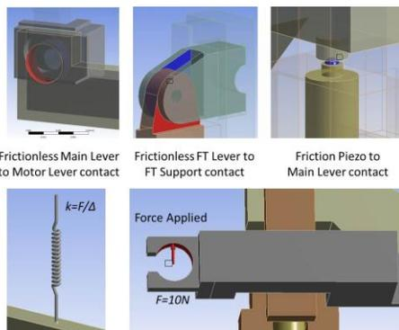
Figure 4: Boundary conditions used in ANSYS analysis.
