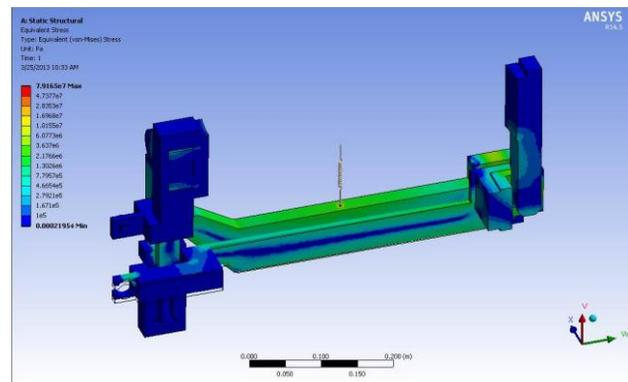
Figure 6: von Mises stresses.
