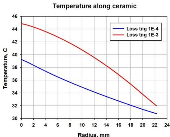
Figure 7: Temperature distribution at the ceramic window. Input power 80 kW, air flow rate 3 g/s.
