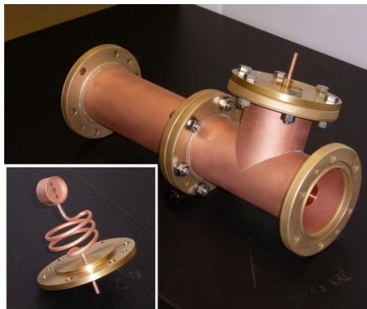
Figure 9: DC block. Tested up to 5.5 kV DC HV.
