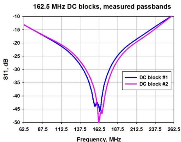
Figure 10: Measured passbands of 162.5 MHz DC blocks.
