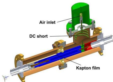
Figure 8: Structure of DC block.
