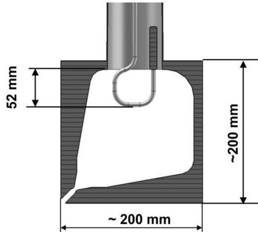
Figure 5: Loop position inside RFQ cavity.
