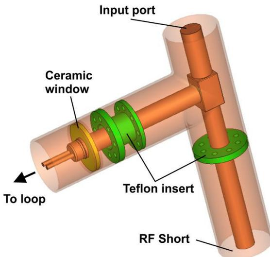
Figure 3: RF structure of RFQ coupler.
