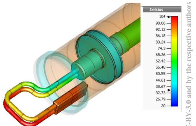
Figure 6: Example of thermal simulations. Input power is 80 kW, air flow rate 3 g/s.
