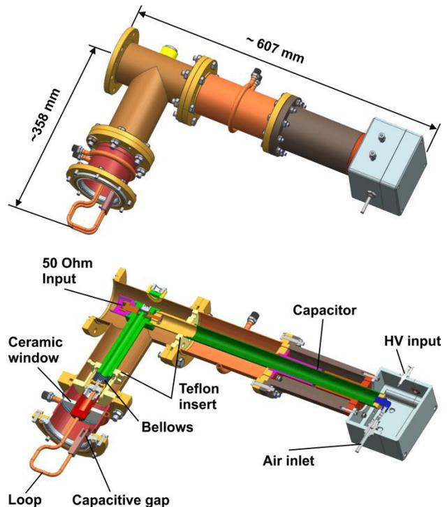
Figure 2: Main dimensions and internal structure of RFQ coupler.
