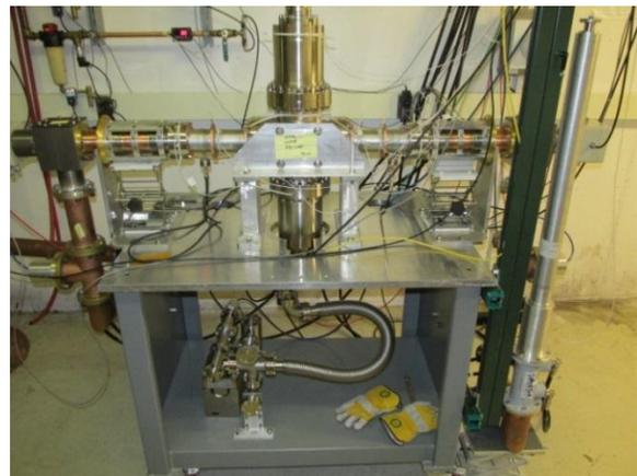
Figure 8: Full assembly of test cavity with couplers ready for testing.
