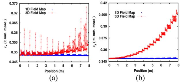
Figure 4: (a) Horizontal and (b) vertical emittance growth without (blue) and with (red) coupler RF kick in HL section for Fermilab type configuration.
