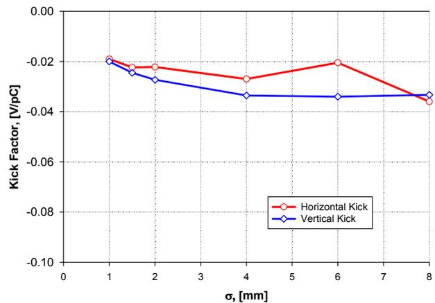
Figure 8: Horizontal (red) and vertical (blue) on-axis coupler wake kick factor in 3.9 GHz cavity.
