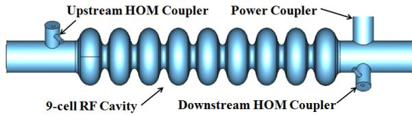
Figure 2: Third harmonic cavity with power and HOM couplers.
