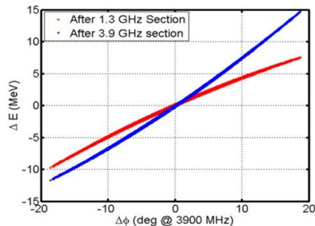
Figure 1: Longitudinal phase space before (red) and after (blue) third harmonic section of LCLS-II SC linac.
