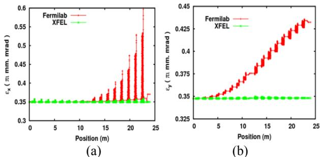
Figure 7: (a) Horizontal and (b) vertical emittance growth in HL section for Fermilab (red) and XFEL (green) configuration of 8 cavity cryomodule.
