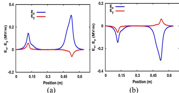
Figure 5: On axis transverse electric fields in a 3.9 GHz cavity for (a) nominal orientation and (b) 180° rotation along the z axis.
