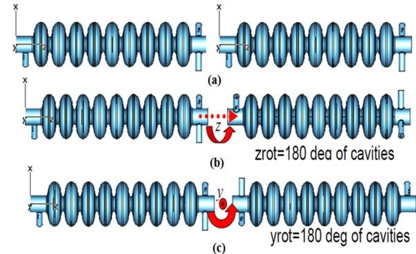
Figure 3: Configuration of cryomodules on the basis of orientation of adjacent cavities: (a) Fermilab type configuration, (b) XFEL type configuration and (c) FLASH type configuration.
