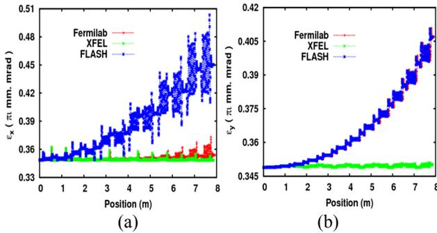
Figure 6: (a) Horizontal and (b) vertical emittance growth in HL section for Fermilab (red), FLASH (blue) and XFEL (green) configuration of cryomodule.
