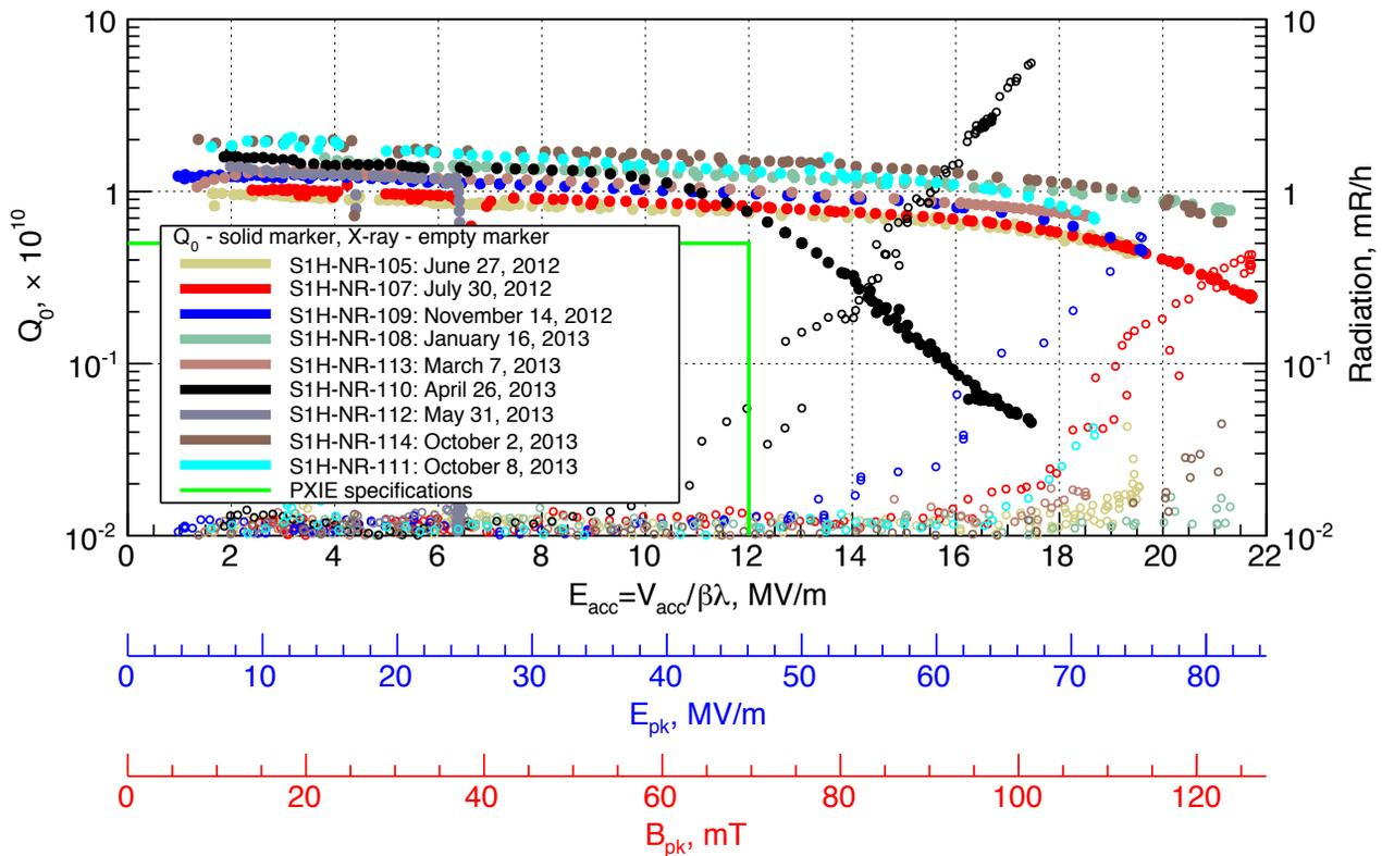
Figure 3: Summary of results of SSR1 cavity tests at 2K.
