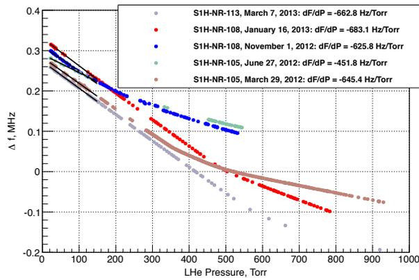
Figure 2: Measurement of the resonance frequency shift vs LHe bath pressure during cool-down from 4.4 K to 2 K.
