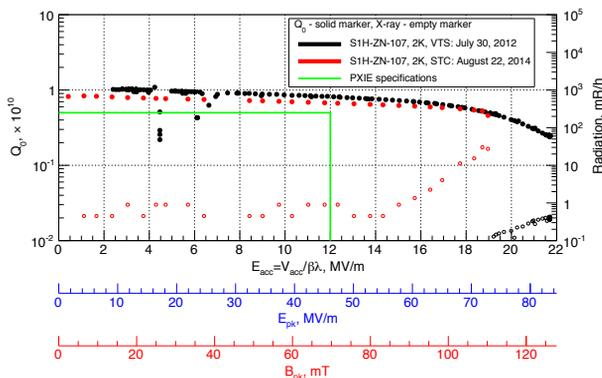
Figure 4:  $Q_0$  and radiation vs  $E_{acc}$  measured at STC.
