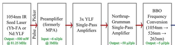
Figure 1: Schematic of the ASTA drive laser system.
