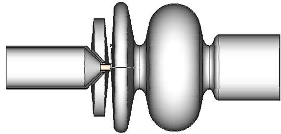
Figure 5: Simulation model of 1.4-cell HZB SRF gun cavity with resonance choke-cell.
