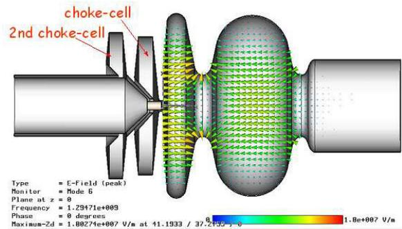
Figure 8: HZB gun option with double choke-cell notch filter.
