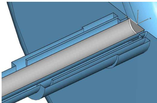
Figure 1: External coaxial quarter-wave length chokes design.
