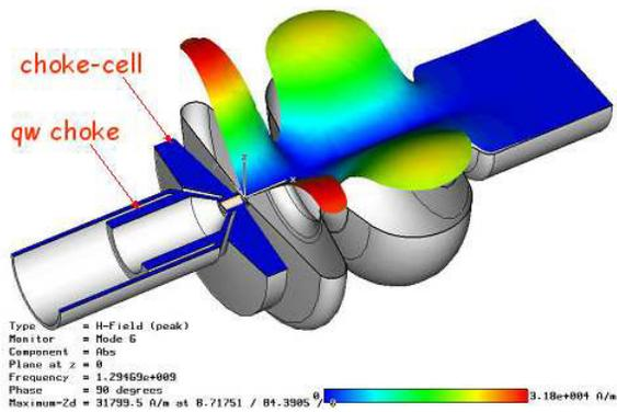
Figure 6: HZB gun option with combined internal quarter wave choke and choke-cell (also magnetic field distribution is shown).
