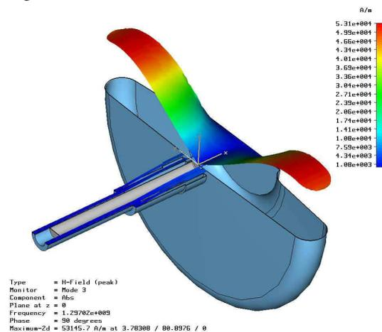
Figure 2: Magnetic field distribution in half-cell and external coaxial quarter-wave length choke.
