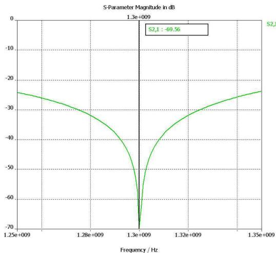
Figure 4: S<sub>21</sub>-parameter of quarter length coaxial choke.
