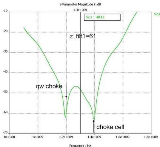
Figure 7:  $S_{21}$ -parameter of the combined notch filter.
