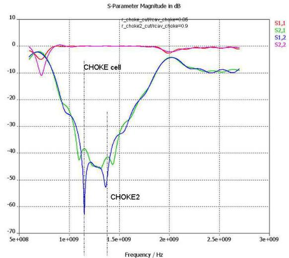
Figure 9: S-parameters of the double choke-cell notch filter.
