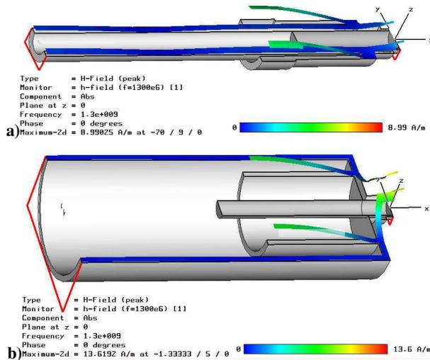
Figure 3: Magnetic field distribution in a) external and b) internal coaxial quarter-wave length choke.
