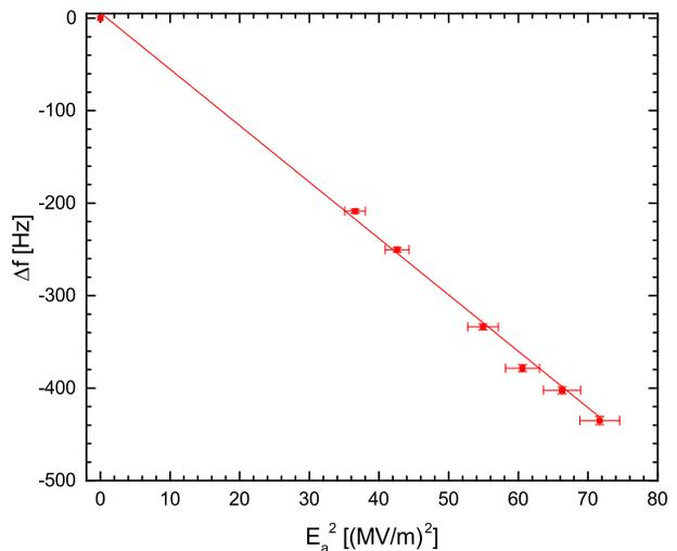
Figure 9: Frequency deviation due to Lorentz-Force-Detuning.
