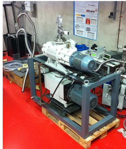
Figure 4: Roots pump for the 2 K setup.
