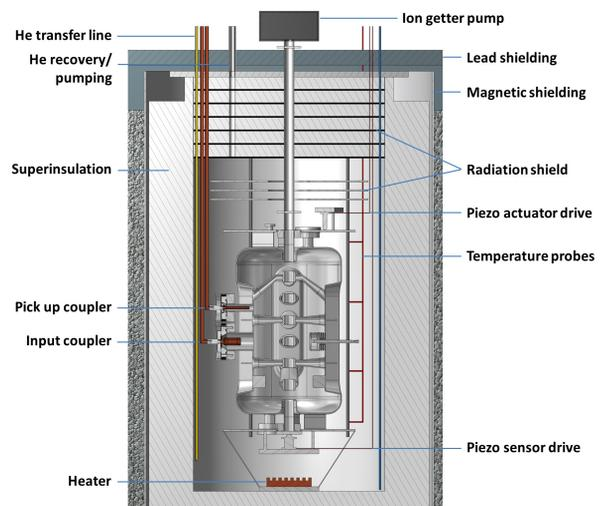
Figure 1: Schematic layout of the vertical cryostat setup.
