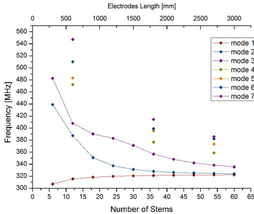
Figure 3: Simulation of the frequency of the higher order modes of a 325 MHz RFQ with increasing electrodes length and stem numbers.
