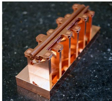
Figure 5: The 6 stem 325 MHz 4-rod copper prototype.
