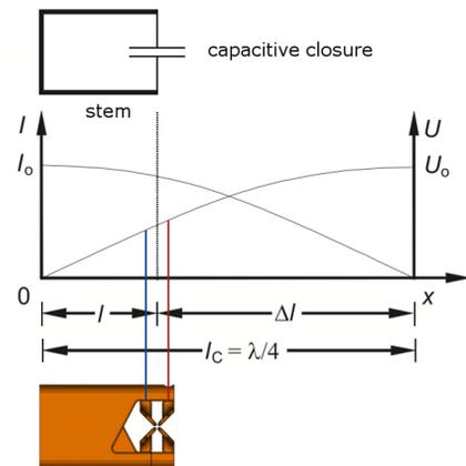
Figure 1: Comparison of a 4-rod RFQ with capacitively shortened Lecher wires.
