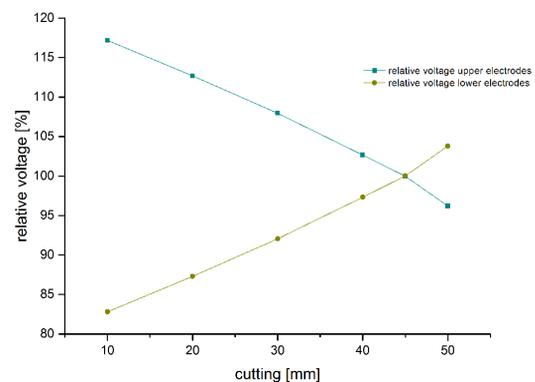
Figure 2: Adjustment and overcompensation of the dipole field by the variation of the angular cutting.
