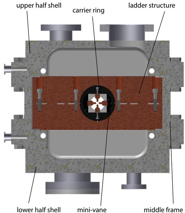
Figure 1: Sectional view through the ladder-structure. The copper carrier-rings (for a better view coloured in black) guarantee the electrode positioning as well as the RF contact.
