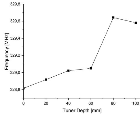
Figure 7: Frequency in dependence of the penetration depth of both parallel driven plungers into cell two and nine.
