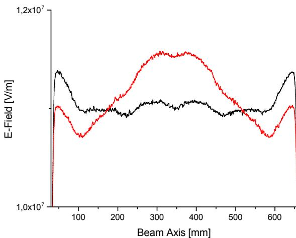
Figure 5: Simulated electric quadrupole field distribution along the beam axis. The red curve shows the distribution with 10 identical ladder cells and the black curve after the adjustment of the width of the end cells. The maximum relative difference of the electric field can hereby be optimized to less than 5%.
