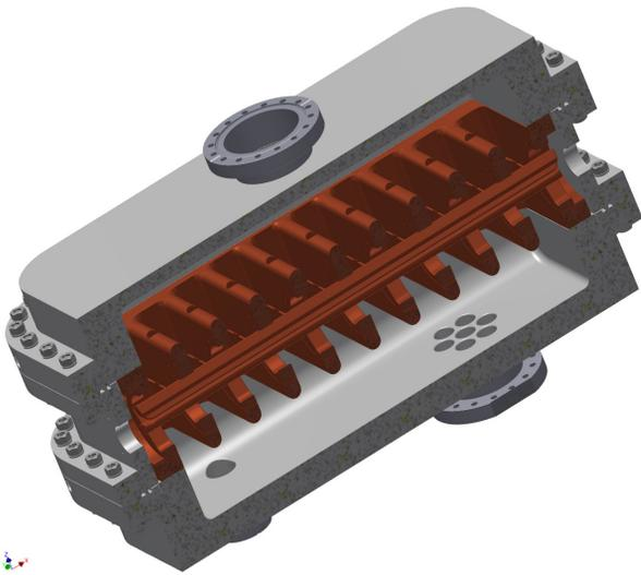
Figure 2: Isometric drawing of the Prototype RFQ. The ladder structure consists of bulk copper components. Any brazing or welding processes are avoided.
