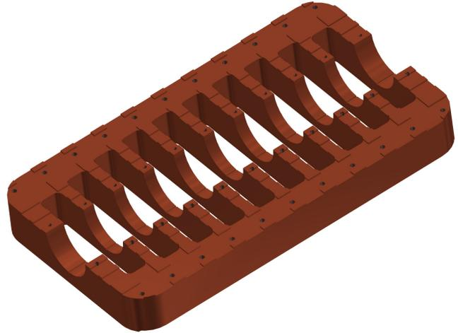
Figure 4: Isometric view of the lower copper shell.
