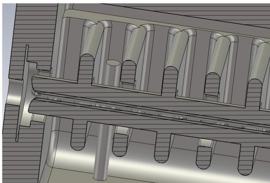
Figure 6: Inductive plunger penetrating the second cell.
