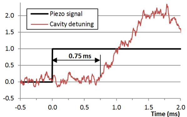
Figure 11: Detuning measurement (phase detection) normalized to the final square wave response value.
