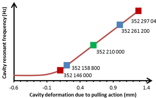
Figure 4: Slow tuner range specification, the green dot represents the nominal set point and the blue dots indicate nominal range of operation. Red dots are ultimate value of operation.
