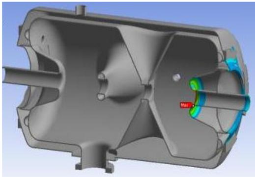
Figure 3: Cavity simulation determined 1.28 mm maximum deformation [1].
