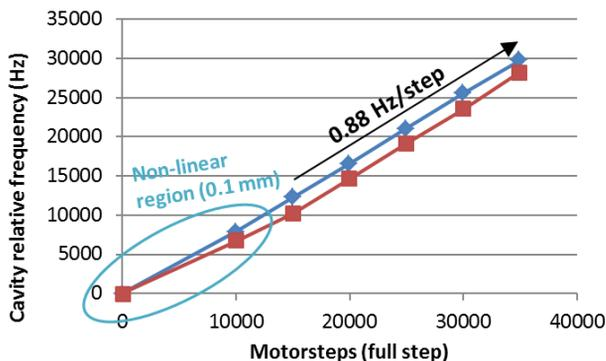
Figure 5: Cavity resonant frequency versus motor action,
