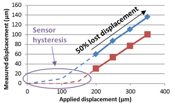
Figure 6: Displacement measurement over limited tuner range, one curve per tuner tested.
