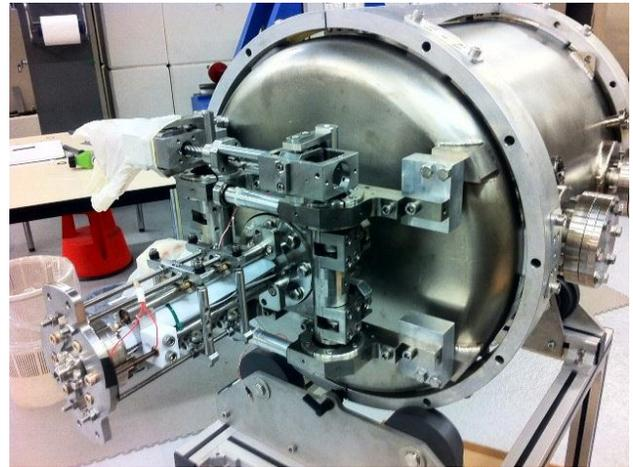
Figure 2: Photo of the tuner assembled on a triple spoke cavity.
