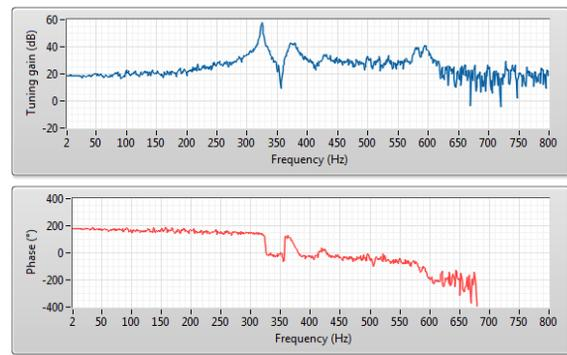
Figure 10: Tuner transfer function, the gain corresponds to the cavity detuning over dual piezo excitation (Hz/V).
