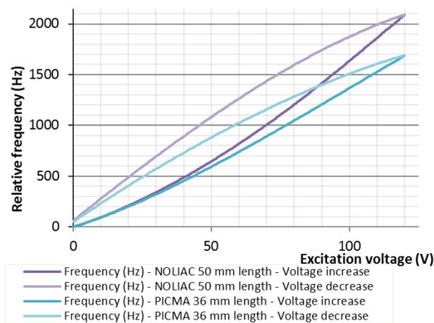
Figure 9: Fast tuner range measurement.
