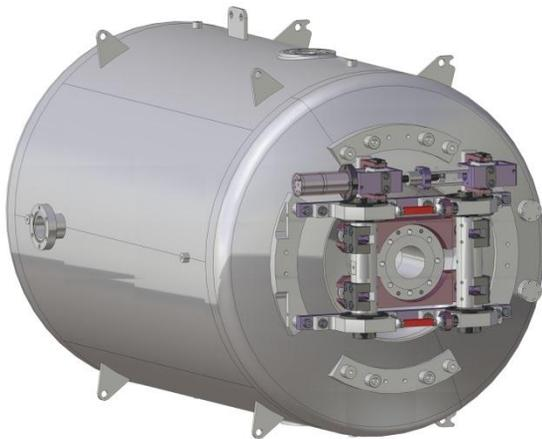
Figure 1: View of the tuner equipping the ESS double spoke cavity.
