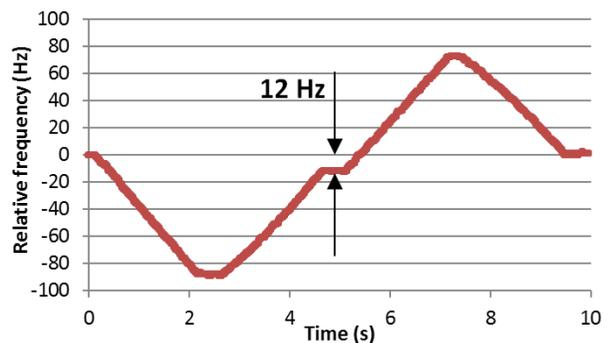
Figure 7: Cavity resonant frequency shift over a very slow and small motor motion of twice 1 µm amplitude.
