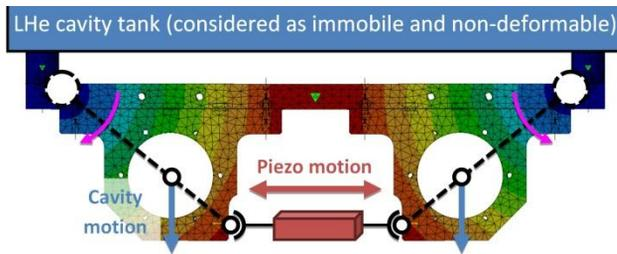
Figure 8: Displacement vector simulation result when the piezo actuators are solicited: red field points the highest value while blue field means no motion.
