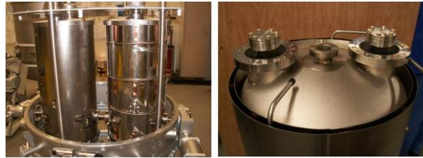
Figure 4: (left): magnetic shield fully assembled (left cavity) and with only one layer and cooling pipe. (right): magnetic shield installed on cavity without the top cover.
