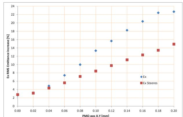
Figure 4: Ex RMS emittance growth without and with Steeres using uniform distribution as input.
