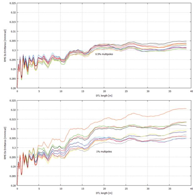
Figure 3: RMS output emittance Ex, due to the multipoles components including the dipoles.
