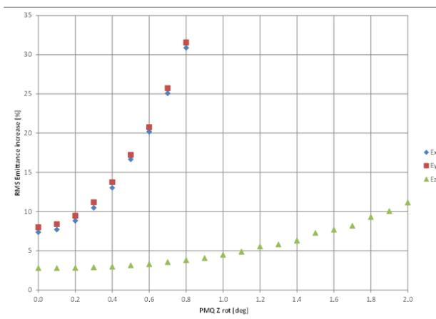
Figure 2: RMS emittance growth, due to the PMQ rotation along the beam axe roll angle.
