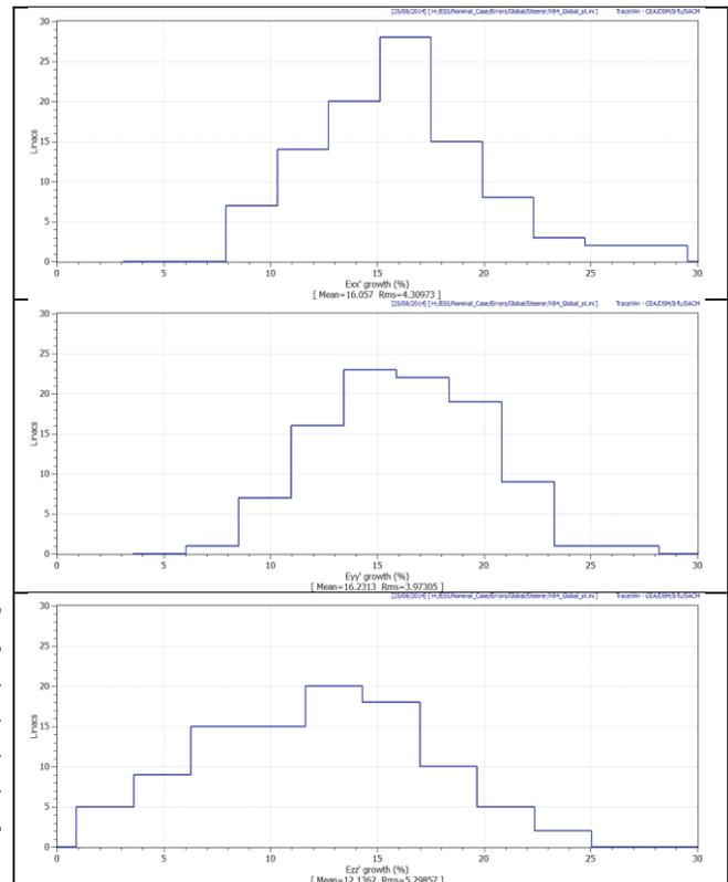
Figure 5: Statistical RMS emittance growth, for the global errors study, with steeres, all runs are without losses.
