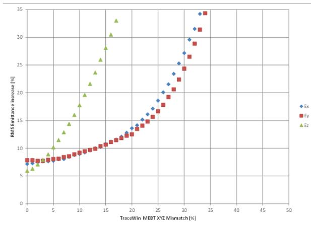
Figure 1: RMS emittance growth, due to the MEBT mismatch on all the planes.
