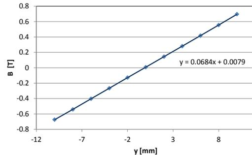
Figure 8: PMQ gradient (Hall probe measurement).
