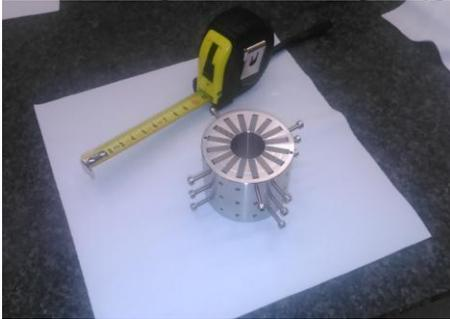
Figure 7: The PMQ prototype.
