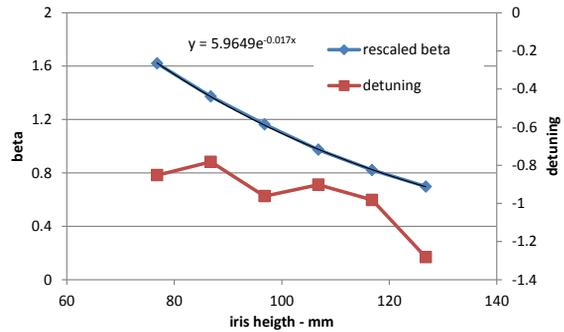
Figure 5: β vs. iris height (iris aperture =70mm).
