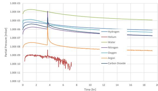
Figure 9: PMQ vacuum test.
