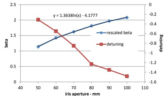
Figure 6: β vs. iris aperture (iris height = 76.8mm).
