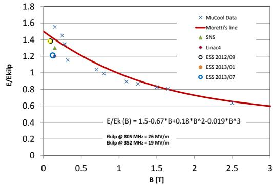
Figure 4: The 1<sup>st</sup> cell of the 2013's ESS DTL is below the breakdown limit curve.
