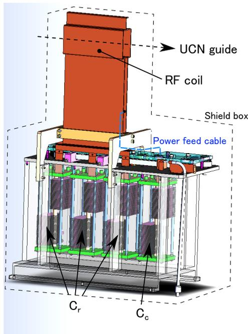
Figure 4: The compositions in the RF cavity of the modified rebuncher.
