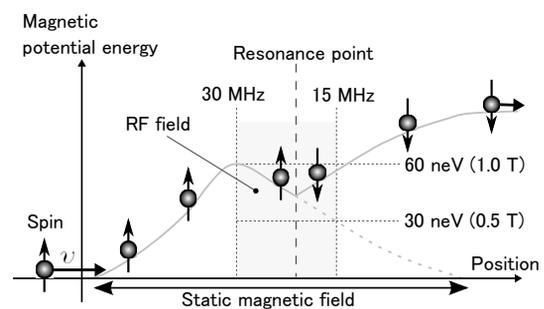
Figure 1: The principle of the neutron acceleration.
