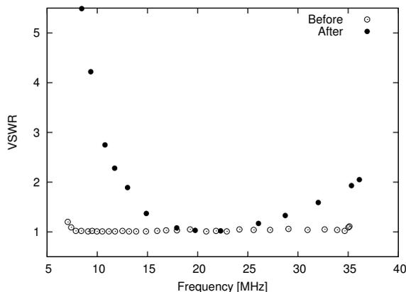
Figure 5: The VSWR before and after modification. The white dots are before modification and the black dots are after.
