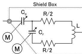
Figure 3: The RF circuits of the UCN rebuncher.
