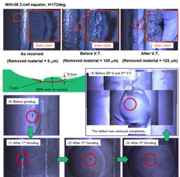
Figure 3: Example of local repair: MHI-08.
