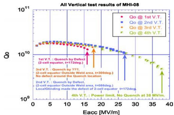
Figure 4: The Q-slope curves of MHI-08 over the repair.
