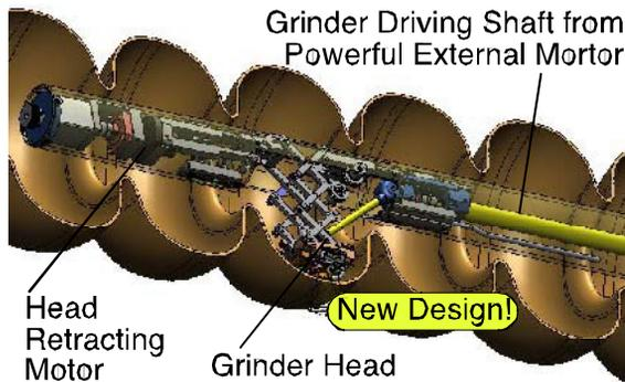
Figure 8: Large external motor delivers more power to the head.
