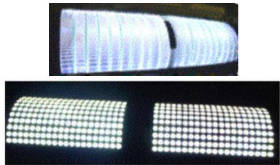
Figure 7: Revised illumination from stripe (top) to dot matrix (bottom). Each dot can be controlled individually.
