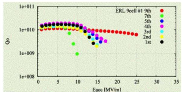
Figure 6: Results on cERL main cavity.
