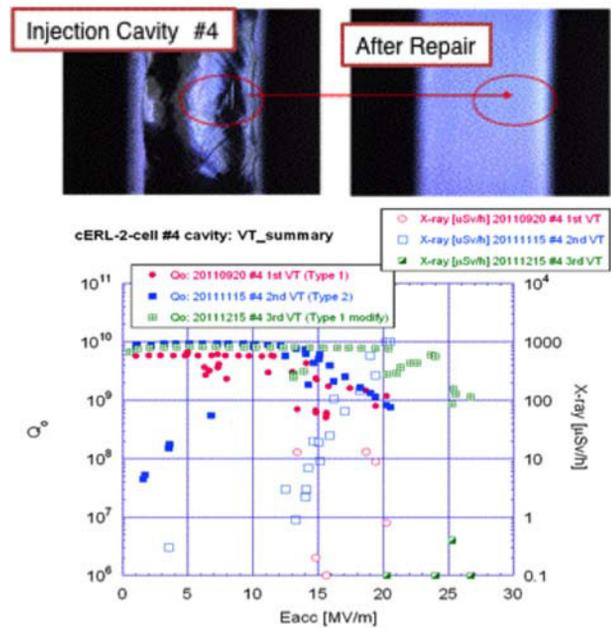
Figure 5: Results on cERL injection cavity.
