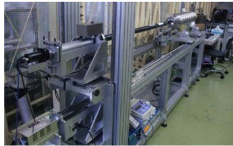
Figure 10: Combined cavity camera and local grinder.
