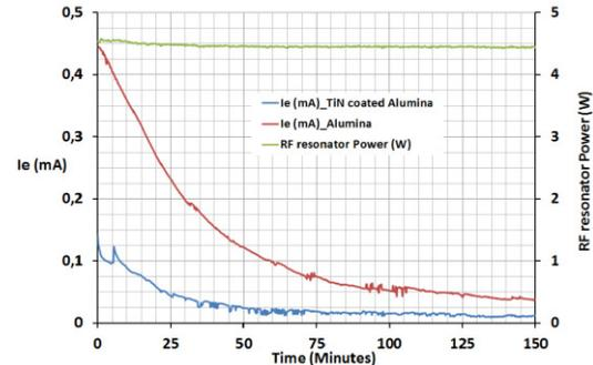
Figure 5: Multipacting current vs. time for 3 different metals.
