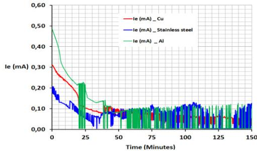
Figure 3: Multipacting current vs. time for 3 different metals.
