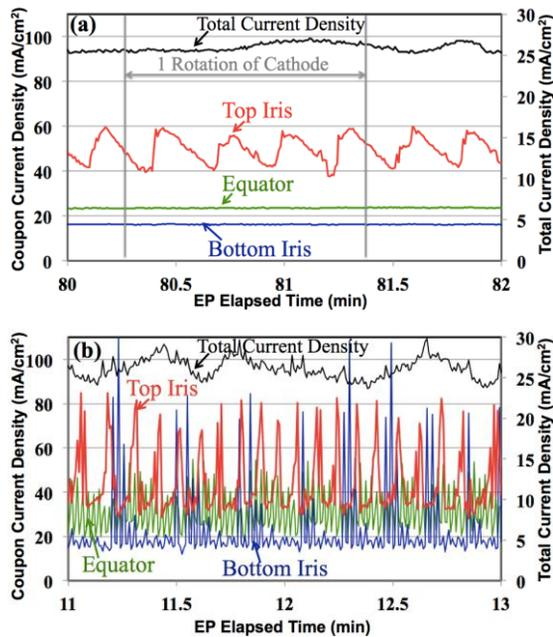
Figure 2: Coupon currents (a) Ninja and (b) rod cathodes.
