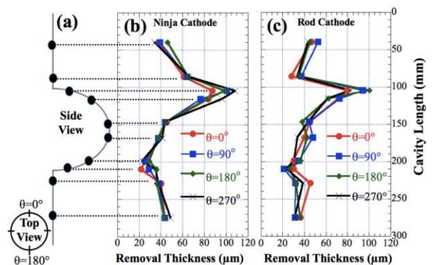
Figure 4: (a) Measuring positions for removal thickness. Measured removal thickness on these positions after VEP with (b) Ninja cathode and (c) rod cathode.
