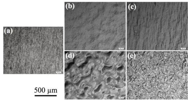
Figure 6: Optical microscope images. (a) Before VEP, (b) Top iris and (c) equator coupons after VEP with Ninja cathode, (d) Top iris and (e) equator coupons after VEP with rod cathode.
