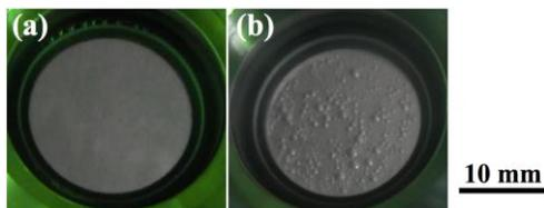
Figure 3: The top iris view port (a) just after passing a wing of the Ninja cathode and (b) rod cathode.
