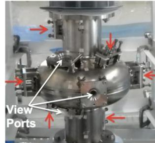
Figure 1: Nb coupon cavity with 6 Nb disk type coupons at beam pipes, irises and an equator shown by arrows.
