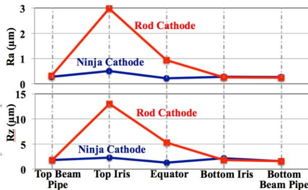
Figure 5: Roughness Ra and Rz of coupons after VEPs.
