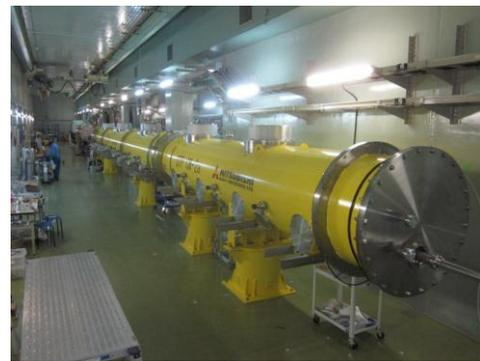
Figure 5: Cryomodule for STF
