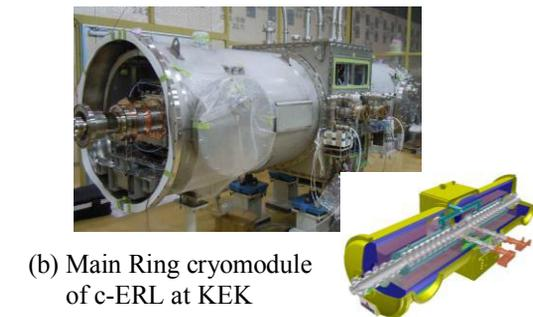
Figure 2: Cryomodules
