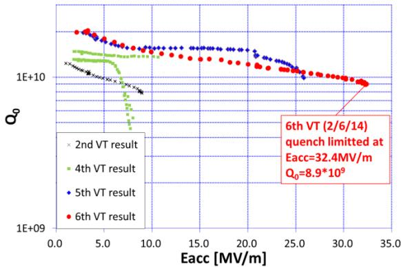
Figure 8: VT result of MHI-B cavity at JLab
