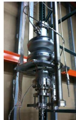
Figure 7: Setting for MHI-B cavity VT
