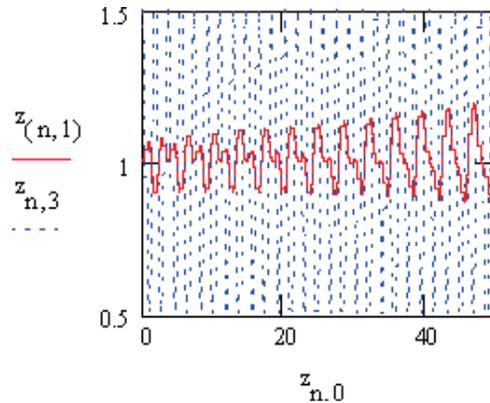
Figure 1: Dimensionless rms radius  $z_{n,1}$  vs dimensionless longitudinal coordinate  $z_{n,0}$  (case of significant deviation of the beam parameters from equilibrium ones)
