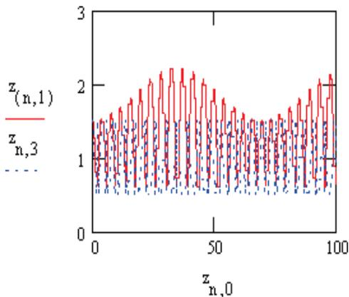
Figure 2: Dimensionless rms radius  $z_{n,1}$  vs dimensionless longitudinal coordinate  $z_{n,0}$  (case of small deviation of the beam parameters from equilibrium ones).
