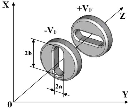
Figure 2: Two-electrode crossed lens
