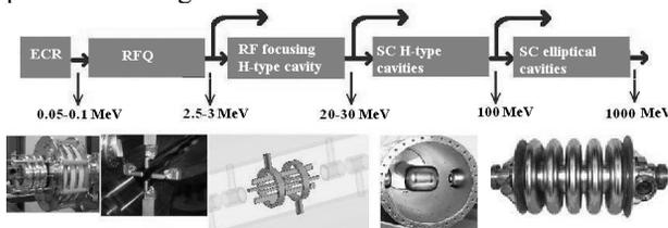
Figure 1: The linac general layout
