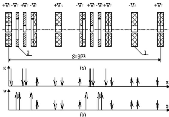
Figure 3: FOODOO focusing period with RF crossed lenses (a) and focusing gradients (b): 1 - round aperture drift tubes; 2 - two-electrode crossed lenses.
