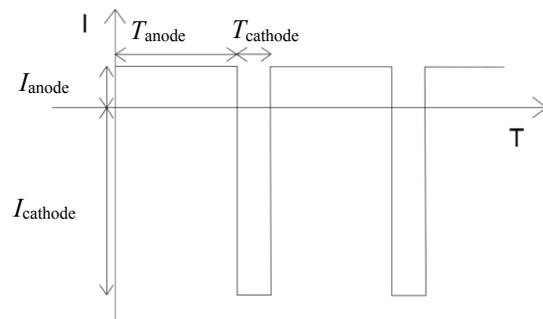
Figure 1: Typical periodic reverse current.
