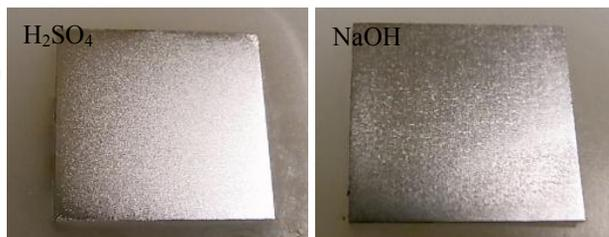
Figure 7: Comparison of the surface of Nb plates by electropolishing with H<sub>2</sub>SO<sub>4</sub> and NaOH solutions.
