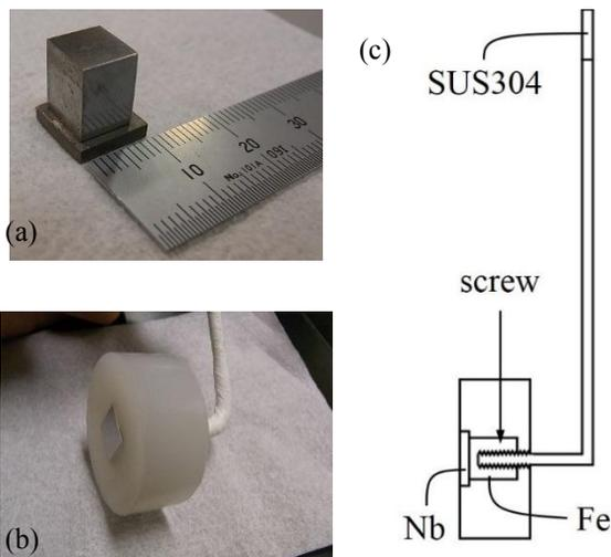
Figure 3: (a) Nb coupon (10 mm x 10 mm x 2 mm) and Fe cube (8 mm x 8 mm x 10 mm). (b) Nb coupon and Fe cube are masked by polyethylene. (c) Schematic of Nb anode with stainless steel (SUS304) rod.
