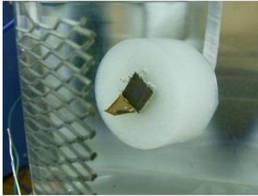
Figure 6: Brown film on the Nb coupon in the Electrolysis with NaOH solution.
