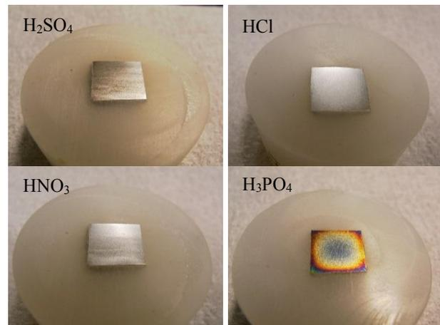
Figure 5: Comparison of surfaces polished with various acids by periodic reverse current electrolysis.
