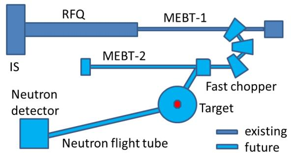
Figure 8: Schematic layout of the ITSF development to include a short pulse neutron source.
