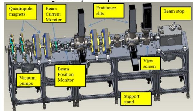
Figure 5: Schematic view of the MEBT and beam stop.
