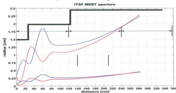
Figure 4: Transverse beam envelope size in the MEBT.
