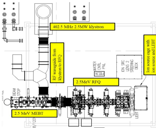
Figure 1: Current layout of the SNS Integrated Test Stand Facility.
