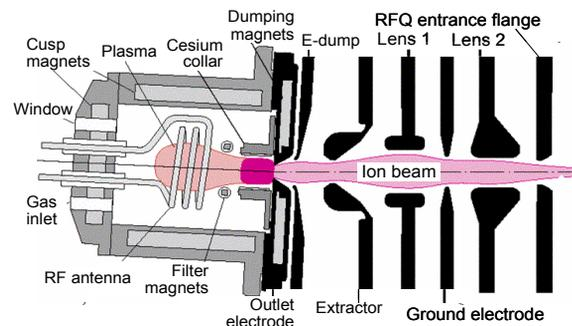
Figure 2: Schematic view of the H<sup>-</sup> ion source and electrostatic LEBT
