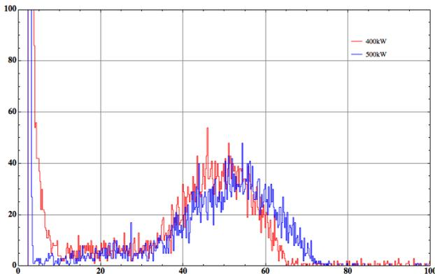
Figure 7: Energy spectra of the X-ray emission from the RFQ cavity measured at different RF power.
