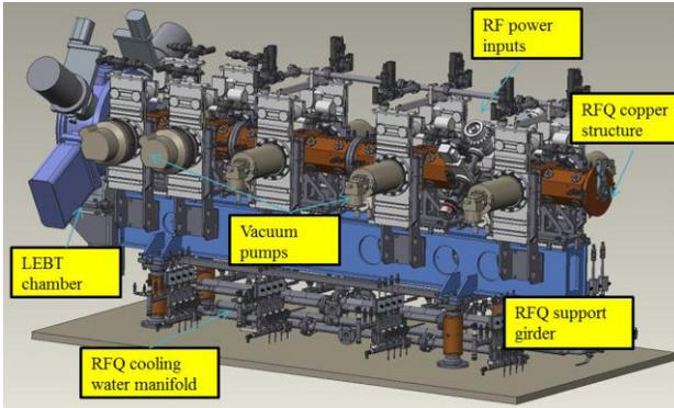
Figure 3: Schematic view of the new SNS RFQ.
